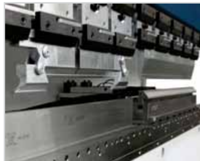
Image 1: tower back gauge BG1T (option) Other configurations are available on request. For different configurations please consult your ADIRA specialist.
