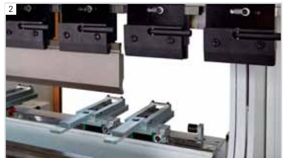
Image 1: tower back gauge BG1T (option) Other configurations are available on request. For different configurations please consult your ADIRA specialist.
